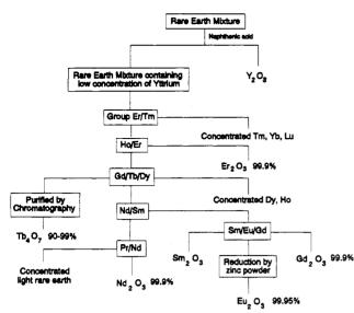
Figure 4. Flow chart of the separation procedure for heavy ore.
