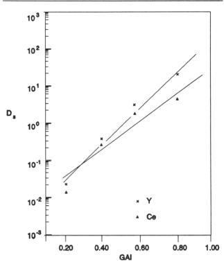
Figure 3. Correlation of GAI and reactivity of Ce and Y with a neutral phosphorus extractant.
