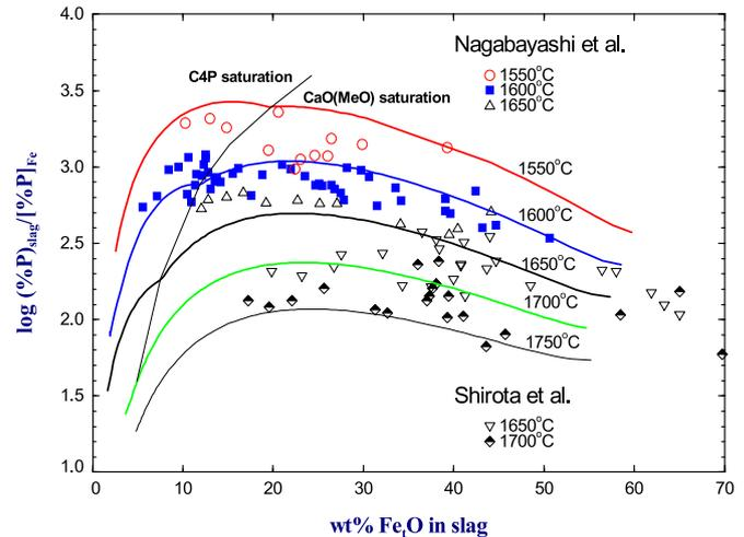
**Fig. 4.** FTOxid database – employed with the FTmisc database to calculate the equilibrium phosphorus distribution between molten slag and liquid Fe as depicted.
