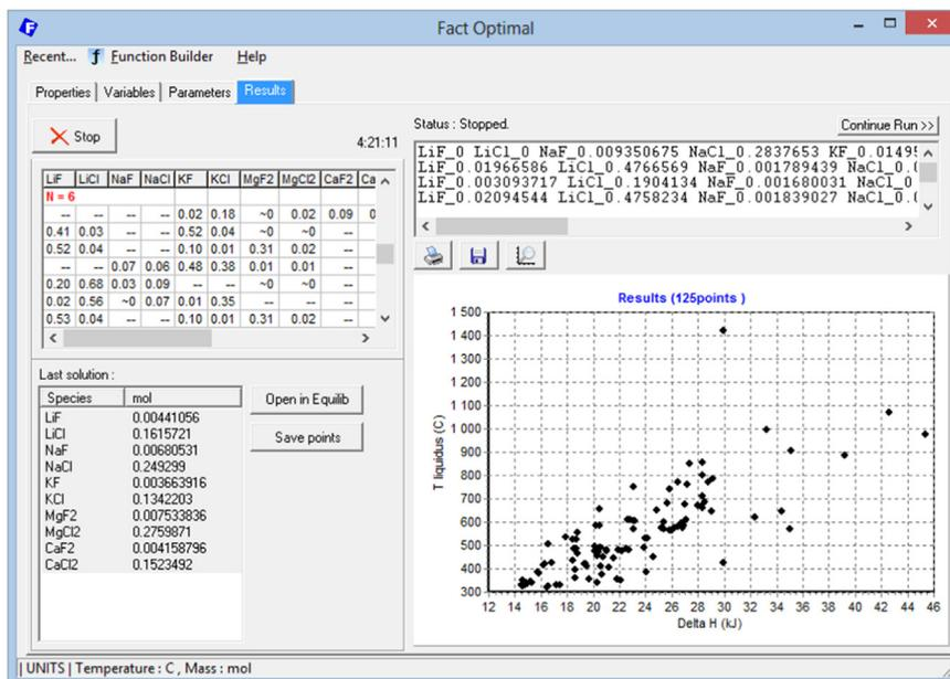
Fig. 16. FactOptimal module – calculated *Characteristic Points* in the  $\text{Li}^+$ ,  $\text{Na}^+$ ,  $\text{K}^+$ ,  $\text{Mg}^{++}$ ,  $\text{Ca}^{++} / \text{F}^-$ ,  $\text{Cl}^-$  reciprocal system.
