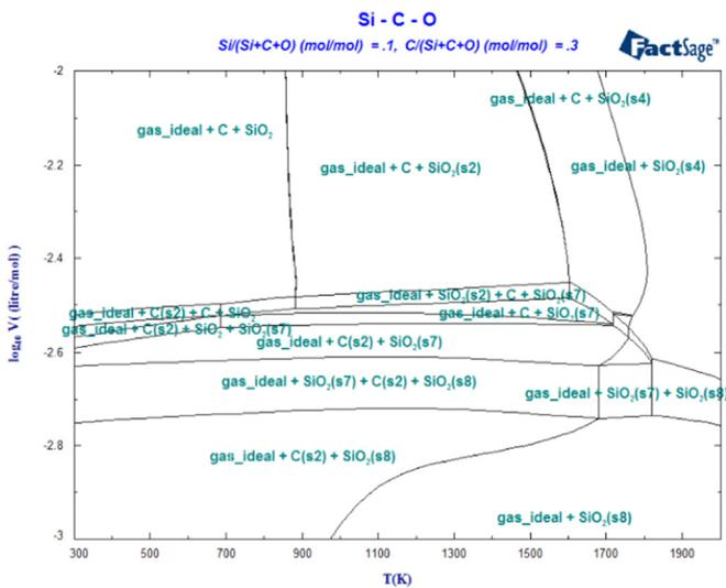
Fig. 26. Phase Diagram – volume diagram of  $\log(V)$  vs.  $T(K)$  in the Si–C–O system when  $\text{Si}/(\text{Si}+\text{C}+\text{O})=0.1$  and  $\text{C}/(\text{Si}+\text{C}+\text{O})=0.3$  (mol/mol).
