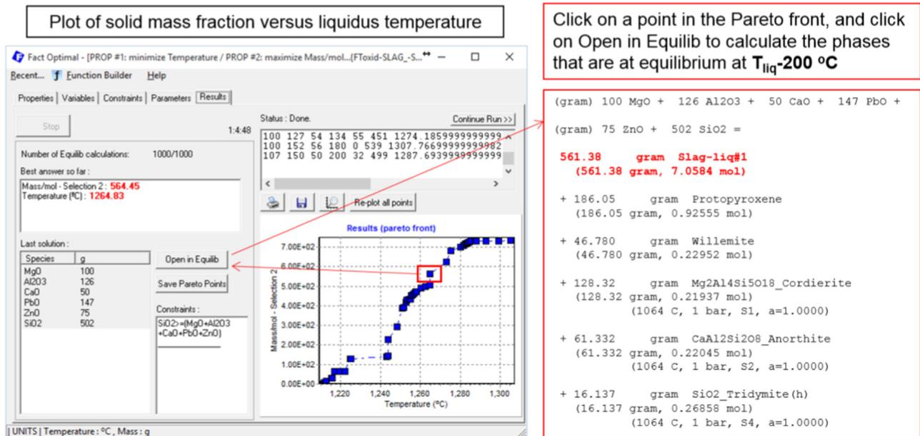
Fig. 17. FactOptimal module – results showing the Pareto front in a plot of solid fraction vs. liquidus temperature in the MgO–Al<sub>2</sub>O<sub>3</sub>–CaO–PbO–ZnO–SiO<sub>2</sub> oxide system.
