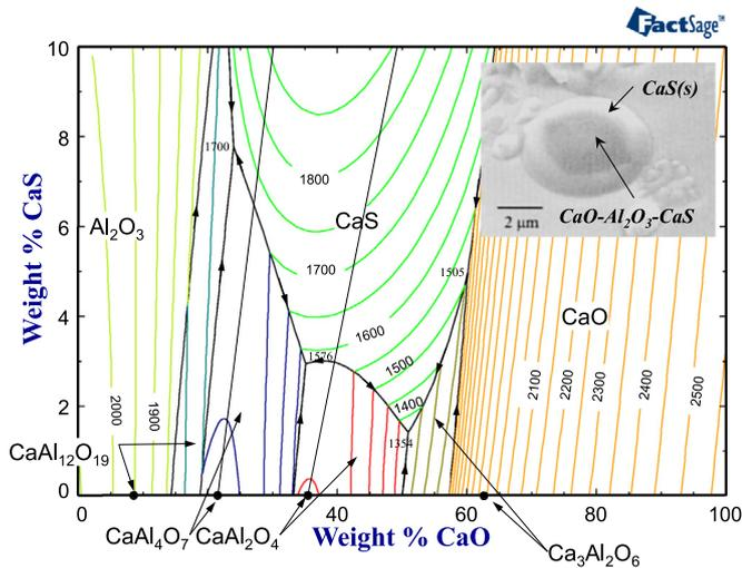
**Fig. 2.** FTOxid database – calculated liquidus projection of CaO–Al<sub>2</sub>O<sub>3</sub>–CaS oxy-sulfide system (FTOxid database) and inclusions found in Al-killed steel followed by Ca injection (inset [4]).
