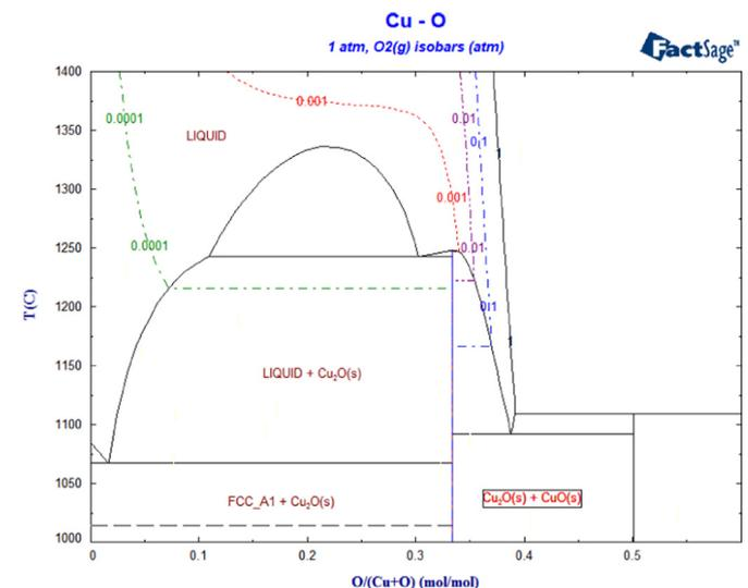
Fig. 34. Phase Diagram module – calculated O<sub>2</sub>(g) isobars in the Cu–O binary systems using data from FSscopp.
