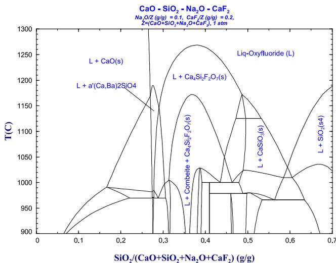
**Fig. 3.** FTOxid database – calculated phase diagram of the CaO–SiO<sub>2</sub>–Na<sub>2</sub>O–CaF<sub>2</sub> system.
