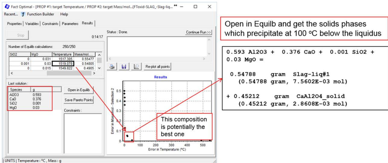
Fig. 18. FactOptimal module – Results Window to minimize simultaneously the liquidus temperature and solid mass fraction in the Al<sub>2</sub>O<sub>3</sub>–CaO–SiO<sub>2</sub>–MgO oxide system.
