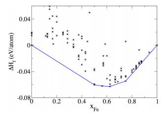
FIG. 2. Example of convex hull stability analysis for Fe-Co alloys, with data points from the AFLOWlib database, used by Troparevsky *et al.*<sup>76</sup> for the purposes of designing high-entropy alloys. Reproduced with permission from Troparevsky *et al.*, JOM **67**, 2350–2363 (2015). Copyright 2015 Springer.
