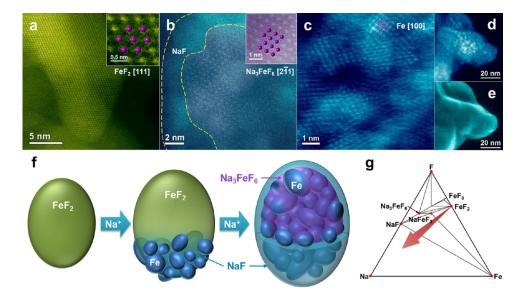
FIG. 3. Information from high resolution STEM images ((a)-(d)) and the computational phase diagram from the Materials Project (g) were employed by He *et al.*<sup>99</sup> to propose a mechanism for sodium incorporation into FeF<sub>2</sub> particles for battery applications. Reprinted with permission from He *et al.*, ACS Nano **8**, 7251–7259 (2014). Copyright 2014 American Chemical Society.
